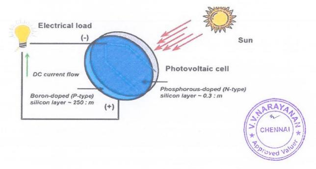
PV cell circuits sealed in an environmentally protective laminate and a solar Module is constructed and are the fundamental building blocks of PV systems. For utility scale, modules will have typically 72 cells.
